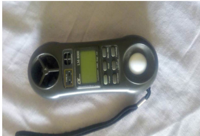
Figure 4: LM 8000 Instrument Measuring Humidity, Air Velocity and Temperature
