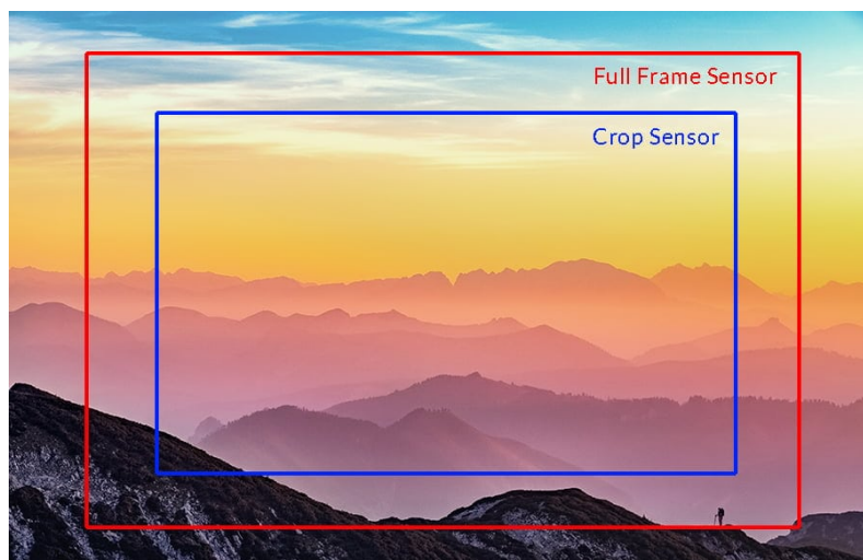
Figure 4. Crop Factor and Depending on Sensor Size
