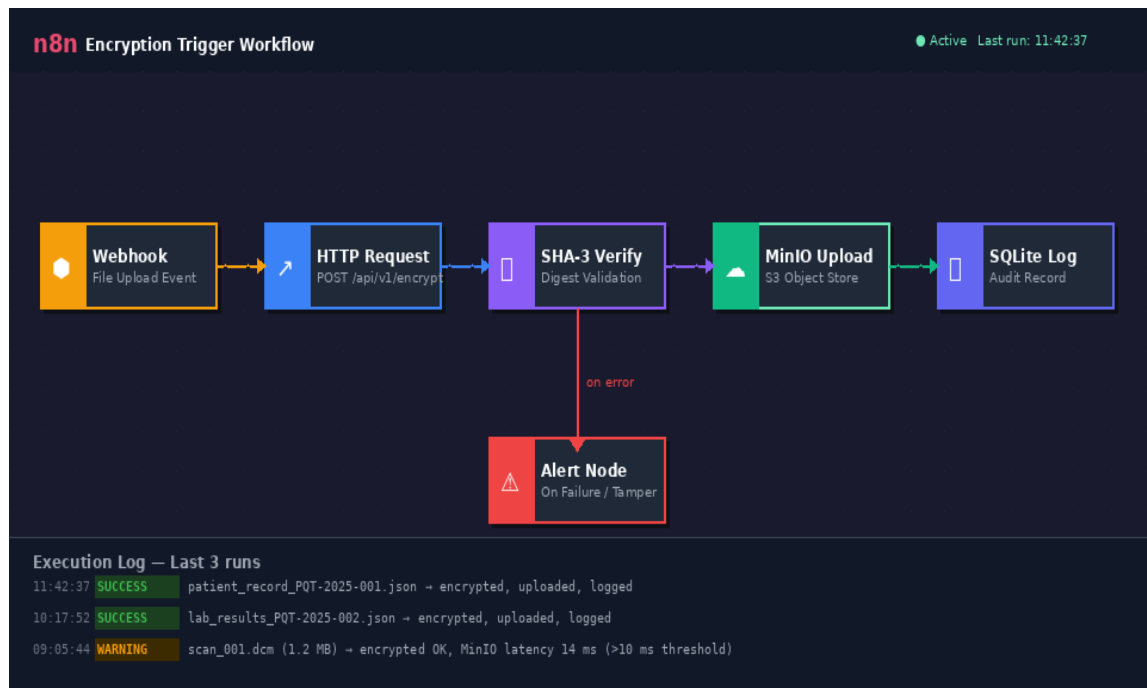
Figure 1. Conceptual architecture of Quantum Shield S3 showing client upload, encryption service, cryptographic engine, MinIO storage, SQLite metadata logging, and n8n workflow automation
